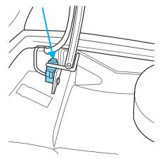
Use the following procedure to reset the fuel pump shut-off switch.
